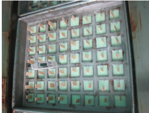
Figure 2. Temperature measurements in the Box with Digital Thermometer
