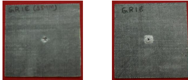
Fig 3.1: Impacted surface & back surface of Graphite /Epoxy Test Specimens after Impact
