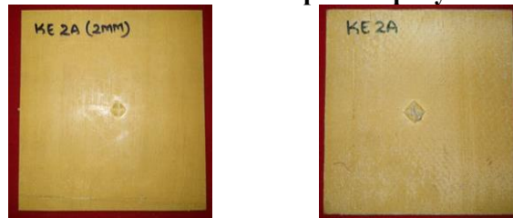
Fig 3.1: Impacted surface & back surface of Graphite /Epoxy Test Specimens after Impact
