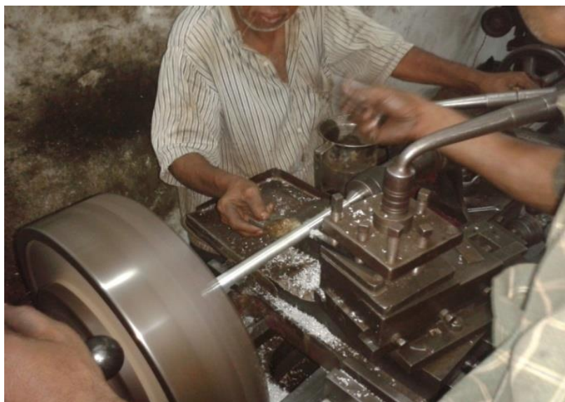
Fig: machining process of casted composite
