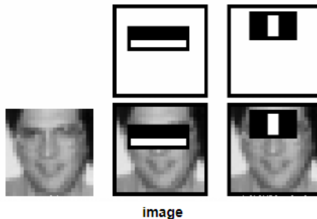
Figure 2: Face Feature extraction classifier
