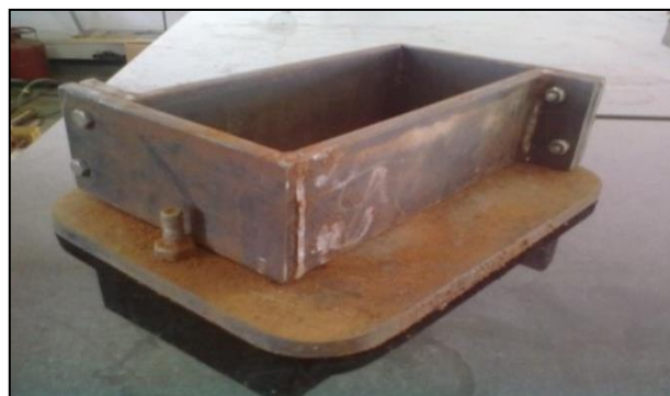
Fig: Mould of size 222 X 106 X 73mm is used to make Recycled Bricks
