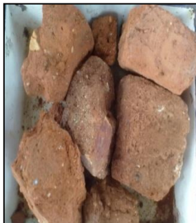
Fig: Demolished Masonry waste and Brick Powder after processing through abrasion testing machine
