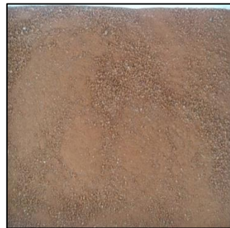
Fig: Demolished Masonry waste and Brick Powder after processing through abrasion testing machine
