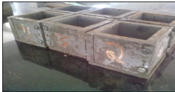
Fig: Cube Moulds (70.6 X 70.6 X 70.6 mm) used to prepare samples
