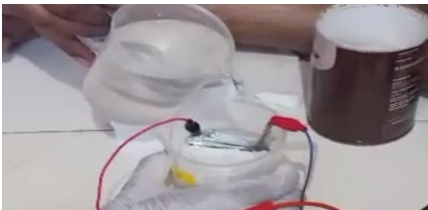
Figure 5: Electrolyte poured into the Aluminium and Activated Charcoal wrapped cell
