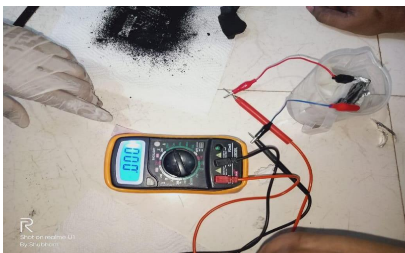
Figure 6: The ready Prototype model of the single cell battery
