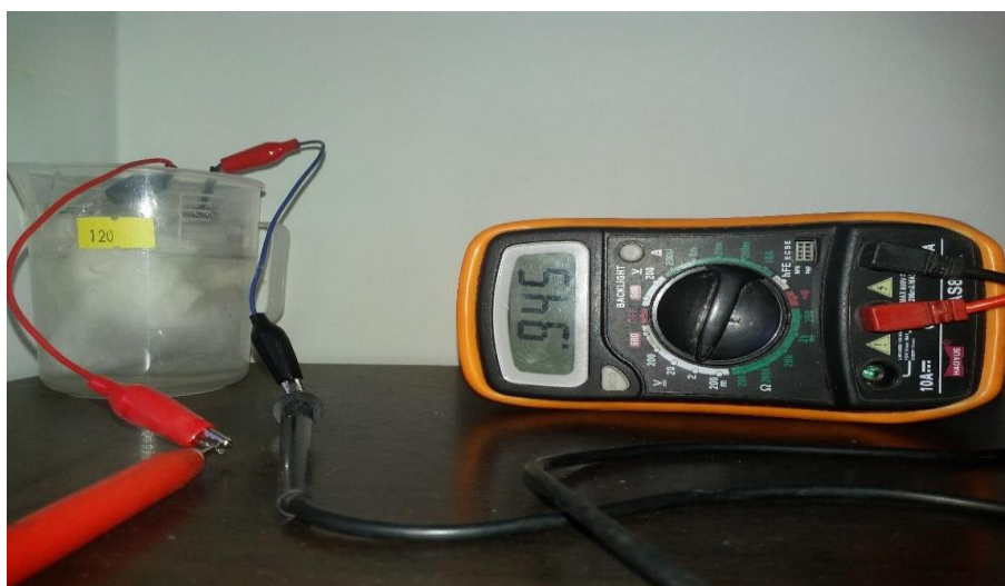
Figure :9 The single cell battery generating 0.945V
