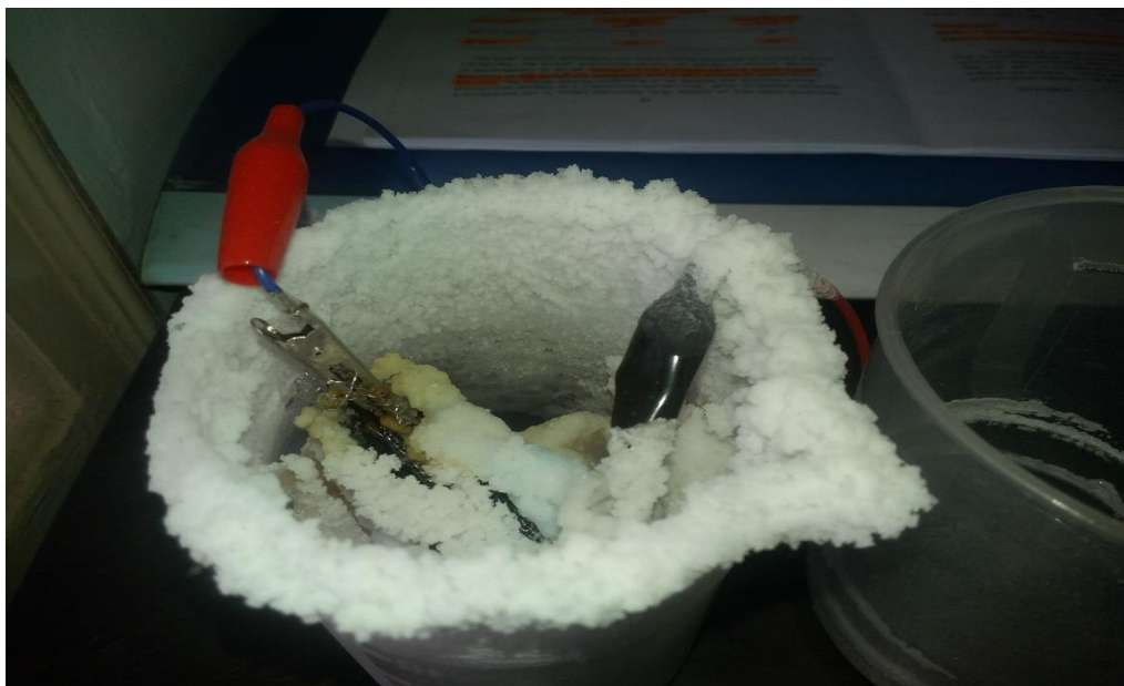
Figure 11: The single cell battery oxidising and developing a layer of salt (after 2 week)
