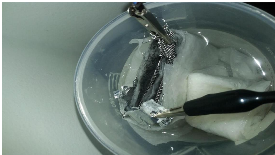
Figure 10: The single cell battery oxidising and developing a layer of salt (after 1 week)
