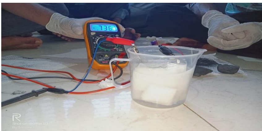
Figure 7: The single cell battery generating 0.736V
