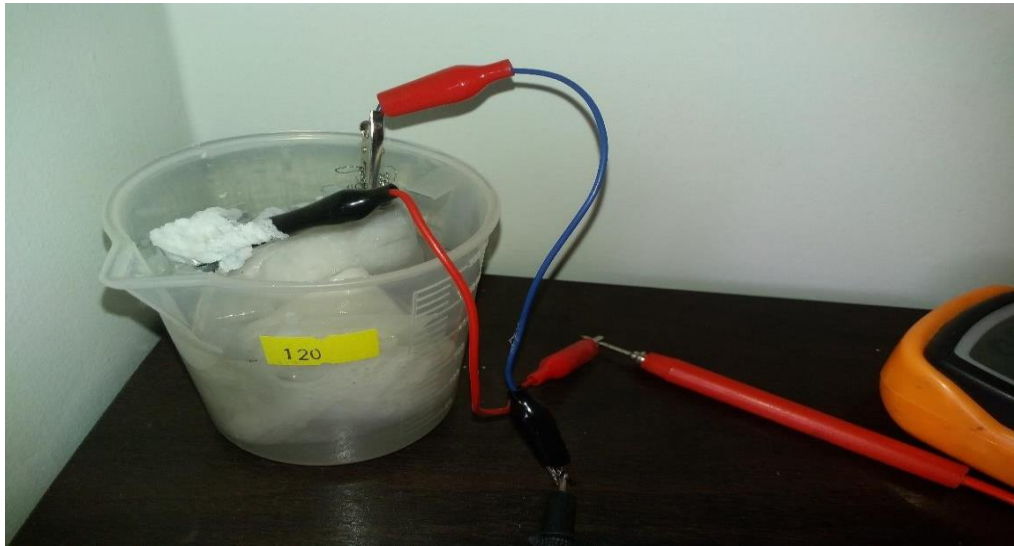
Figure 11: The single cell battery oxidising and developing a layer of salt (after 2 week)
