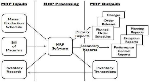
Figure 2: The Function of MRP (B.N.ITAFE 2005)
